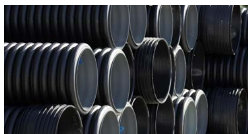
Gaines techniques recyclées ©A.D.I. Valor
